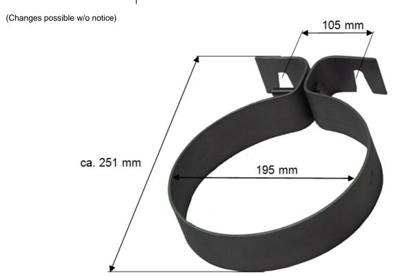
Set of wall mounting brackets (pair) consisting of clamp, each with a hex bolt and hex nut (M10). The clamp is designed for bag filter housings ECOLINE (EBF) and FLOWLINE (FBF) sizes 01 and 02 and allows wall mounting.
