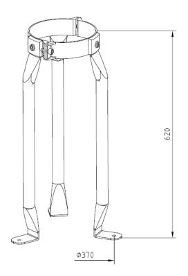
Two-piece leg assembly made of a two leg clamp and a one leg clamp. For fixing the leg assembly to the bottom you find three 10 mm drills. With this height adjustable leg assembly you can fix the vessel in the needed height.
