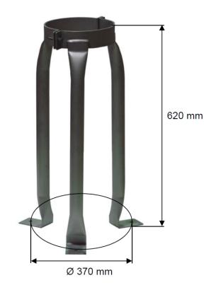
Two-piece leg assembly made of a two leg clamp and a one leg clamp. For fixing the leg assembly to the bottom you find three 10 mm drills. With this height adjustable leg assembly you can fix the vessel in the needed height.
