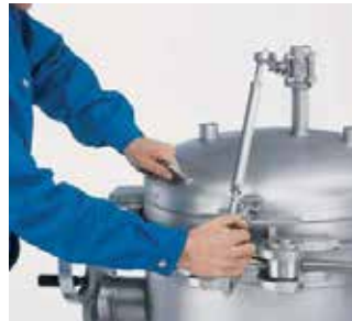
1. Filter element change necessary – open the safety interlock to ensure simultaneous pressure relief.
