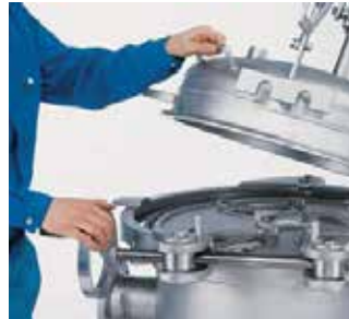
3. Open the cover aided by spring-assisted mechanism.
