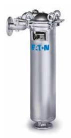
TOPLINE single bag filter housing is simply the best—from its high-performance design to its investment-cast components. The top inlet design requires less headroom and directs liquid flow through the cover which improves sealing, reduces product loss and makes filter bag change-outs cleaner. ASME coded.
