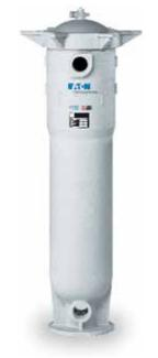
POLYLINE single bag filter housing is constructed with glass fiber reinforced polypropylene or PVDF. It features superior corrosion resistance as well as high-pressure and temperature capabilities. The POLYINE has one injection molded body meaning no seams or weak points.
