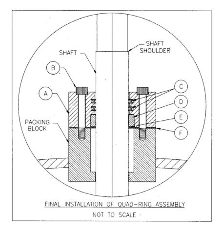
9. Polish Shaft from top of Packing Block to Shaft Shoulder with Crocus Cloth provided.
