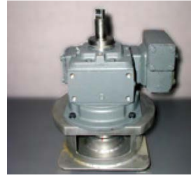
Photo 12: After the idL™ bearing seal is in place, the gear reducer is replaced on the top of the strainer.
