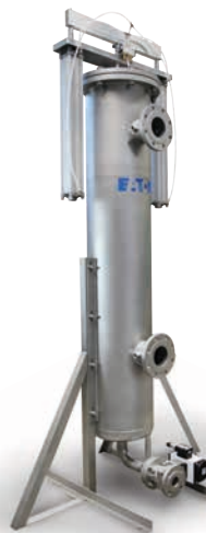
DCF-3000 - This dual cleaning disc and twin actuator design is ideal for highly viscous, abrasive or sticky liquids with flow rates of up to 500 gpm. For water-like liquids, it can handle flow rates up to 1500 gpm.
