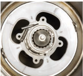
Eaton's unique spring-loaded cleaning disc (shown here in an MCS-500) ensures precise contact with the filtration screen to thoroughly and uniformly clean the media.
