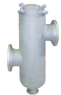
Eaton's Model 90 fabricated simplex strainer ranges from 1" to 48" in pipeline size and can be ordered in carbon steel, stainless steel or other specified materials. The Model 90 offers an in-line design featuring ANSI Class 150, 300, or 600 flange connections. Higher pressures are also available.
