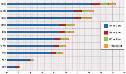
Dirt-holding capacity according to ISO 16889 (test dust: ISO-MTD) of different filter media and filtration grades. Dirt-holding capacities at 29, 58, 87, 116 psi (2, 4, 6, 8 bar) pressure differential.
