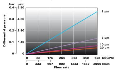
\* For liquids other than water, multiply pressure drop by fluid viscosity in centipoise.
