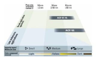
The activated carbon of the BECO MiniCap ACF filter is a microporous, inert material with a very large inner surface of up to 2000 m<sup>2</sup>/g of activated carbon. The activated carbon used can be divided into different porosity ranges:
