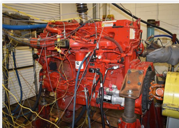
FIGURE 2 Cummins X15 engine platform installed in test cell.
