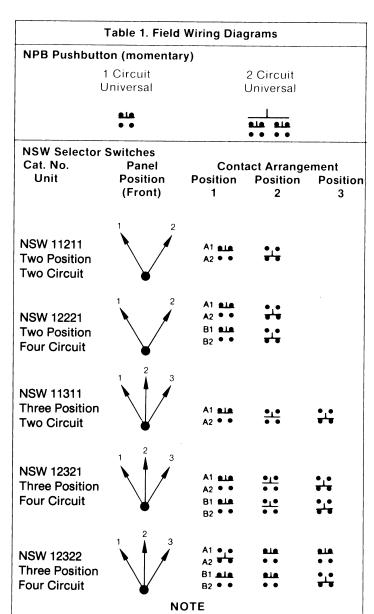
For three-position selector switches with suffix S634, Position 3 is momentary contact with spring return to Position 2. For three-position selector switches with suffix S635, Position 1 is momentary contact with spring return to Position 2.
