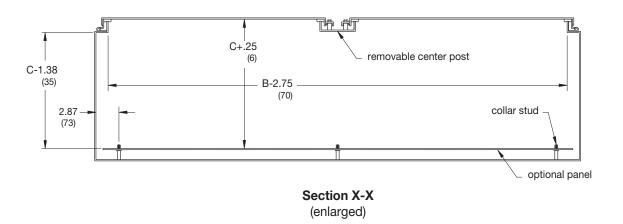
Notes: Clamps are mounted along three sides of the enclosure door. Spacing between clamps along side opposite the hinge does not exceed 15 inches. Four lifting eyes are furnished when C dimension is 24". Dimensions are in inches. Millimeters shown are for reference only. Data subject to change without notice.
