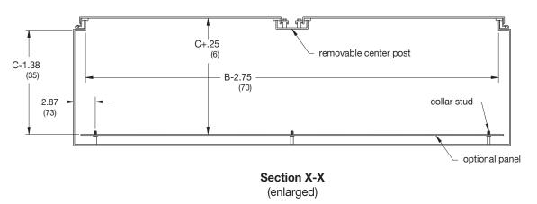
Notes: Clamps are mounted along three sides of the enclosure door. Spacing between clamps along side opposite the hinge does not exceed 15 inches. Four lifting eyes are furnished when C dimension is 24". Mounting legs shipped unassembled on aluminum enclosures.
