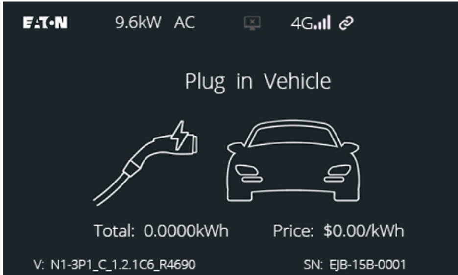
Figure 10. LCD screen of EV charge station connected to Eaton CNM via cellular
