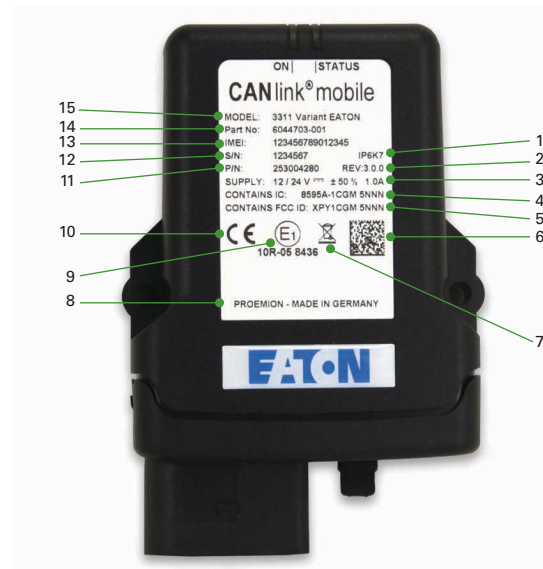
Fig 2. TFX type label (here: model variant TFX internal antenna)
