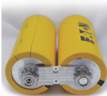
Figure 2: Assembled cell connecting negative terminal on the left to positive terminal on the right.
