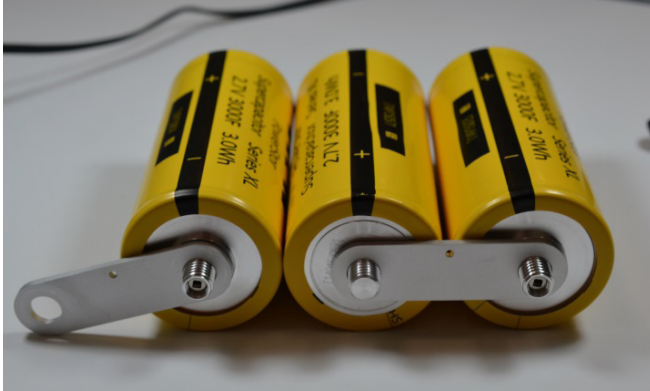
Figure 2. Connect cells in series. Polarity located on the black stripe
