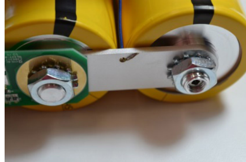
Figure 4a. Insert exposed wire into hole
