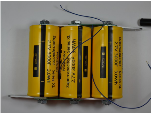
Figure 3. Assembled cells with lock washer and nuts
