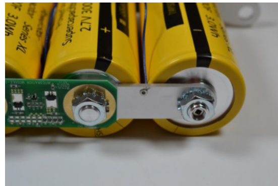
Figure 4c. Rivet per standard riveting procedure
