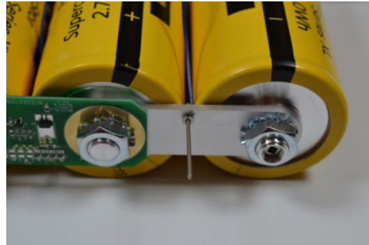
Figure 4b. Insert rivet
