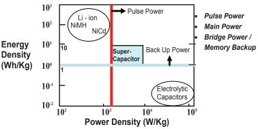
Figure 1. Energy and power density of Supercapacitor, battery, and elctrolytic capaciotrs
