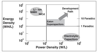
Figure 1. Power density vs. energy density
