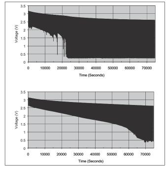
Figure 2. 2 AA alkaline batteries (top) to 2 AA alkaline batteries connected in parallel to a single 6F super-capacitor (bottom)
