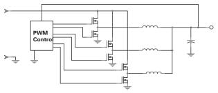
Figure 1. Multi-phase Voltage Regulator Module
