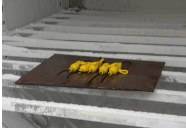
Figure 1. HFB-R with specified wire, installed per specification, tested under IP6x test conditions
