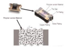
Figure 5. Voltage variable material ESD suppressors
