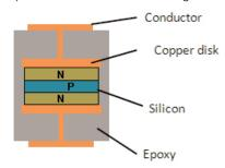
Figure 7. Transient Voltage Suppression construction
