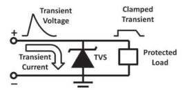
Figure & Transient Voltage Suppression operation
