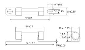
Note: recommended tightening torque is 4.5+/-1.0 Nm for M5 Screw
