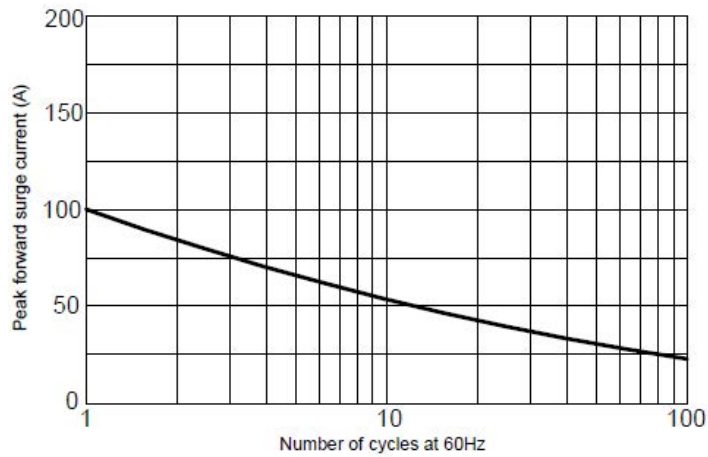
Maximum non-repetitive peak forward surge current (8.3ms single half sine-wave) (+25 °C)
