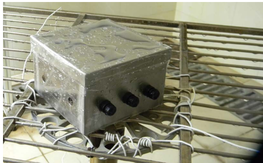
Figure 5. Testing for IP ratings on Eaton's HKP-W-R fuse holders
