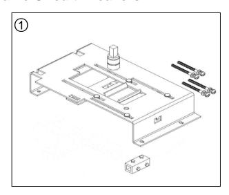
2.2 As shown in Fig. 3, mounting mechanism onto circuit breaker, ensuring slide plate is engaged with the circuit breaker handle. Fix mechanism with washers, lockwashers and screws (1/4-20 x 92) by package supplied. Torque to 5 N.m (44.25 in-lb).
