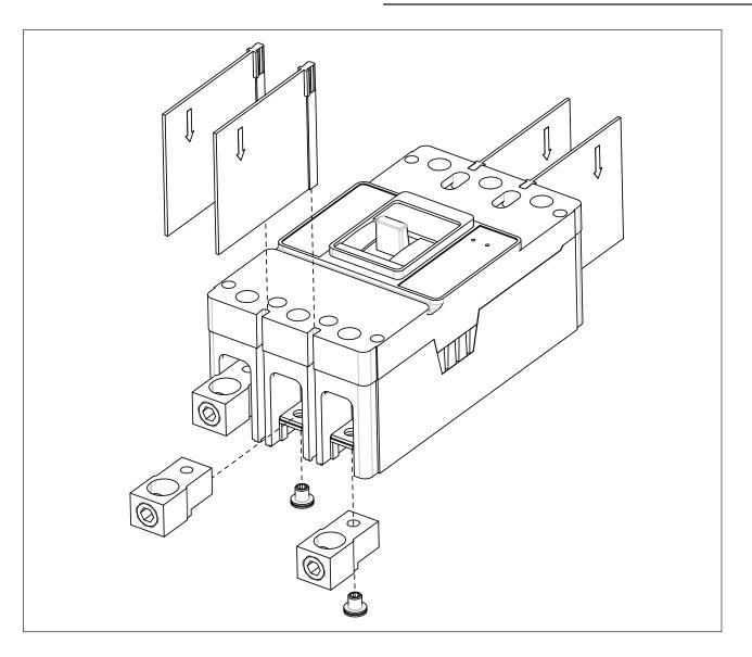
Instructions for K-Frame 500 MCM Terminal Kit, Catalog No. 3TA350KRF. For Use on Series C K-Frame Circuit Breakers, Molded Case Switches, and Motor Circuit Protectors.
