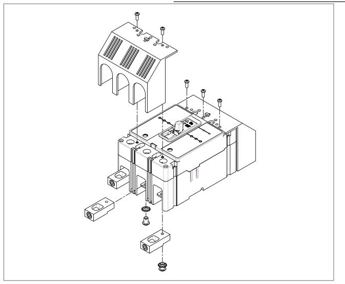
Instructions for F-Frame 4/0 AWG Terminal Kit, Catalog No. 3TA150FDRF. For Use on Series C F-Frame Circuit Breakers, Molded Case Switches, and Motor Circuit Protectors.
