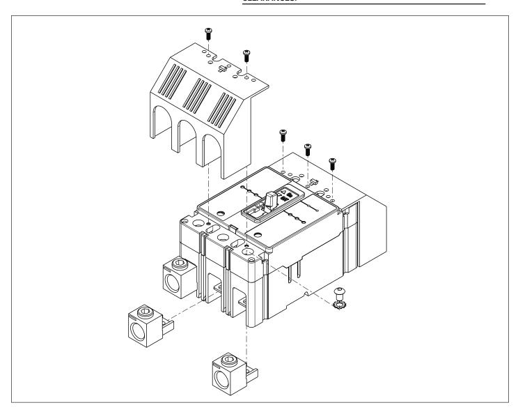
Instructions for F-Frame 300 MCMTerminal Kit, Catalog No. 3TA225FDK3. For Use on Series C F-Frame Circuit Breakers, Molded Case Switches, and Motor Circuit Protectors.
