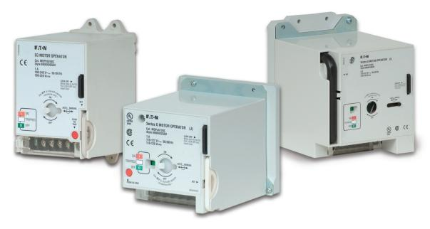
The Eaton motor operator mechanism enables local and remote ON, OFF and reset switching of a circuit breaker. The motor operator is mounted on the circuit breaker cover within the dimensions of the circuit breaker. The robust motor operators offer various voltages to maximize customer flexibility. Standard load transfer switching can be accomplished through the use of two circuit breakers fitted with motor operators and a mechanical interlock.
