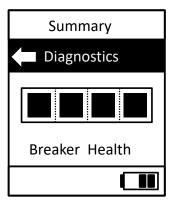
When the summary of life is indicating 25% or less, the breaker should be inspected for possible replacement.
