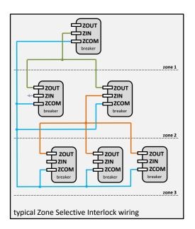
Motor protection circuit breakers are used in the final breaker (lowest zone) in a complete ZSI enabled system. The zone out (Zout) signal is sent whenever a short circuit delay protection or ground fault protection pickup is exceeded. This indicates to the circuit breaker in the zone above that the fault has been seen and will be acted upon. For all motor protection circuit breakers, the zone in (Zin) signal is not used.
