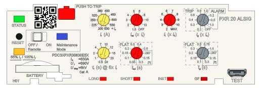
Depending on the trip unit style, up to seven rotary switches can be found on the trip unit's front panel. The switches are color-coded and set protection settings using a surrounding legend indicating the value of that setting. These are the core protection settings, other configurable settings can be set using PXPM. Details regarding the available protection settings for each frame are found in Section 9: Available protection settings.
