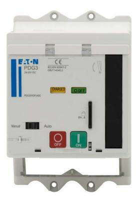
The Eaton Power Defense<sup>™</sup> motor operator enables local and remote ON, OFF and reset switching of a molded case circuit breaker. The motor operator is mounted on the circuit breaker cover within the dimensions of the circuit breaker. The new and improved design offers a wide range of voltages to maximize customer flexibility.
