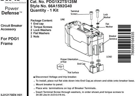
. Place wire terminations on top of Breaker Terminals.
