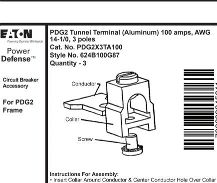
Install Screw to Secure the Collar on the Conductor.
