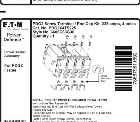
Torque Terminal Screws to 34-38 lb-in (4.0-4.4 N-m).
