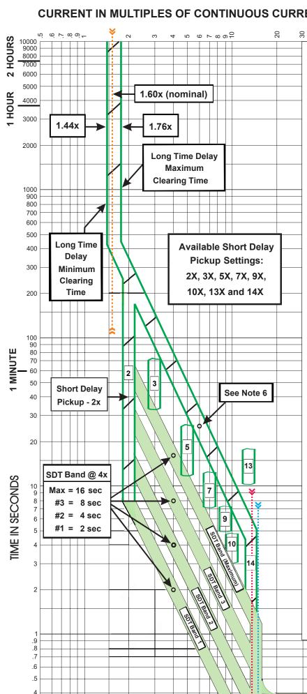
**Circuit Breaker Time / Current Curves (Phase Current)**
