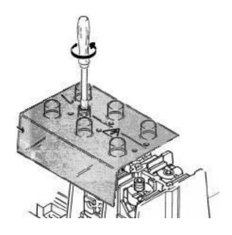
Disconnect the cables from the circuit-breaker
