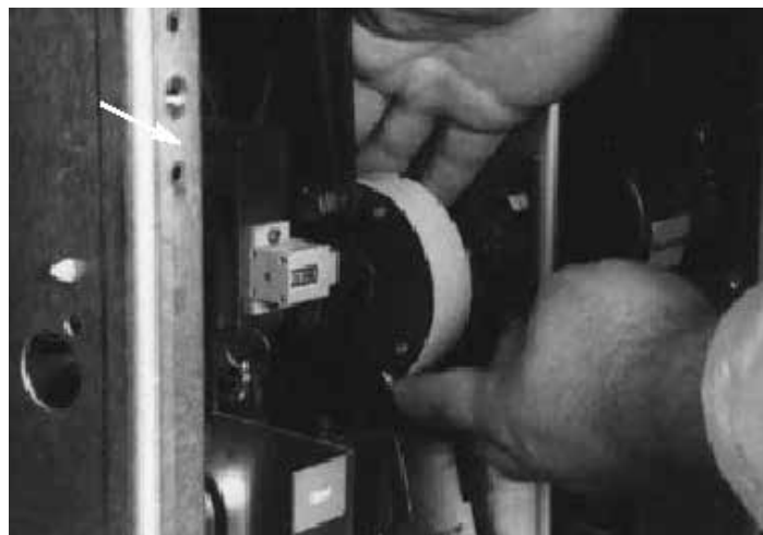
Figure 33. Attaching tape around to the back of the cam.
