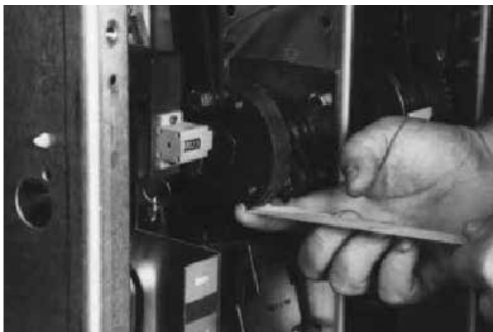
Figure 31. Starting tape at the bottom of the cam.
