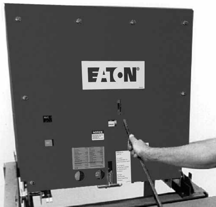
Figure 10. Type VCP-W circuit breaker manual charging handle in use.
