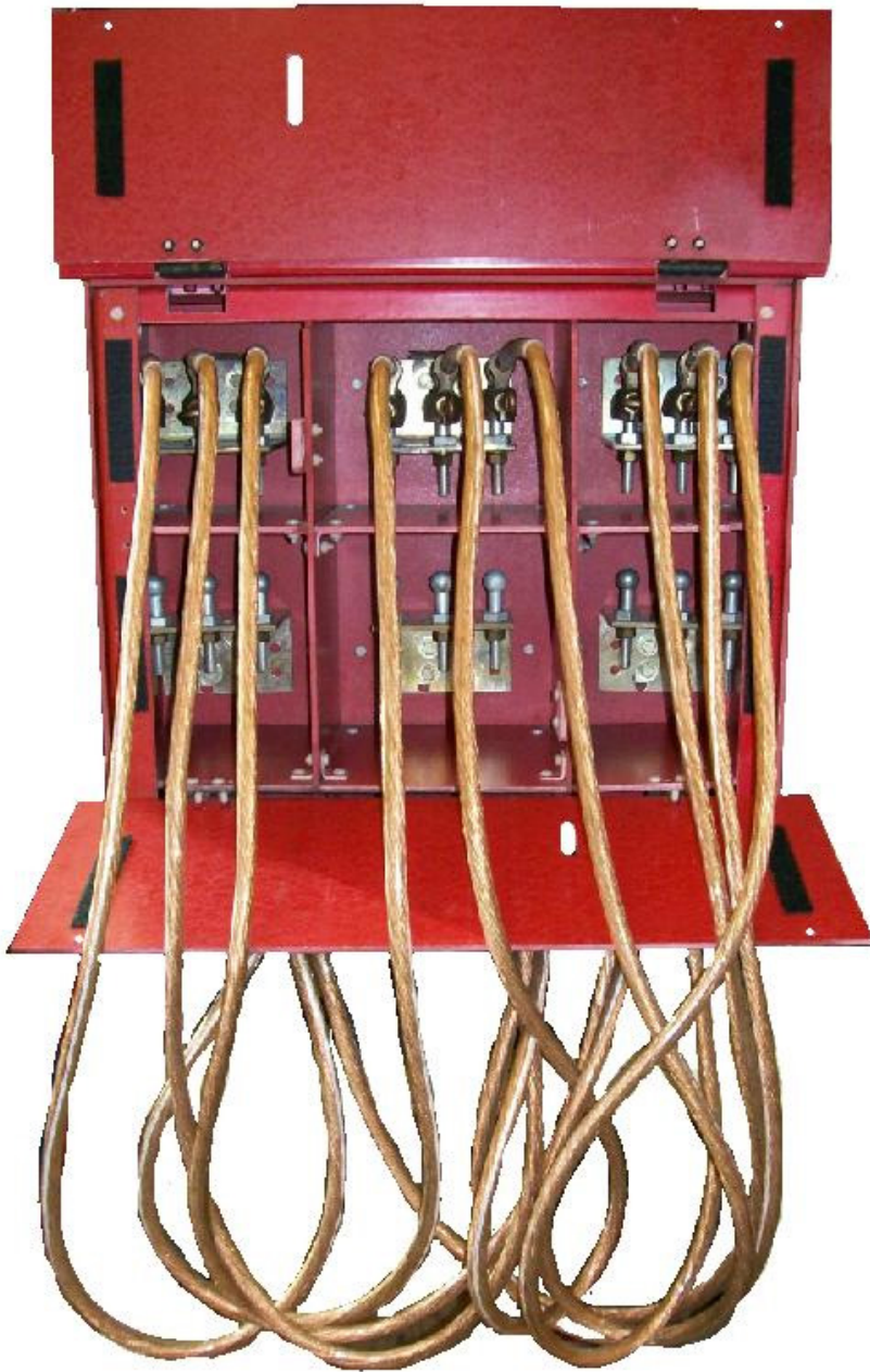
Figure 6: Reference picture of Ball Type Ground & Test Device wired using the three Cable Ground Set (9 total cables). This version is shown with the top terminals connected. The same connection method should be used for a bottom connected system.
