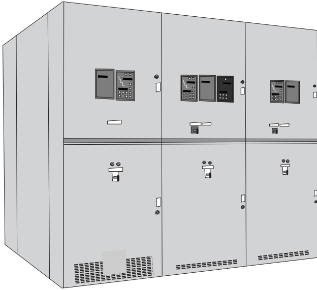
Figure 2 – Typical Switchgear Assembly with Microprocessor-based Protective Relays and Other Devices
