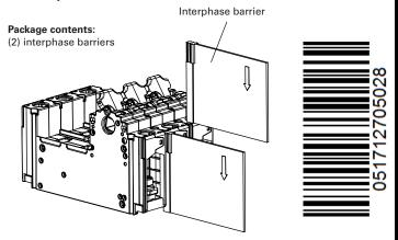
Interphase barriers may be assembled to either lineside or loadside of 2- or 3-pole switches and two or three ganged CUBEFuse holders.
