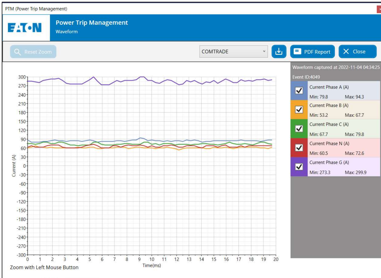
Figure 7.3: Last waveform recorded with COMTRADE format selected
