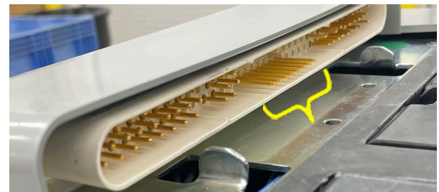
Figure 4. Breaker side secondary connector.
