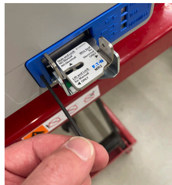
Figure 15. Door latch release hole.
