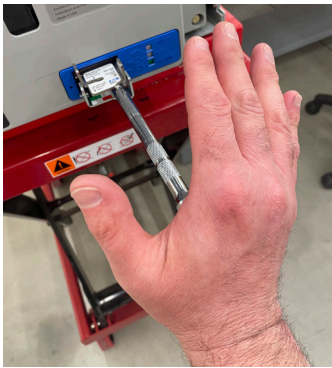
Figure 10. “Un-locking” the clutch.
