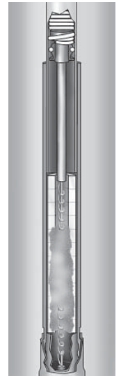
Vapor quenches arc at first current zero
