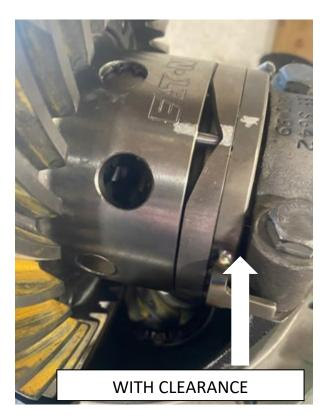
Install the bearing cap bolts and adjuster nut to the manufacture's recommended specifications. Recheck and adjust bearing cap clearance if necessary.
