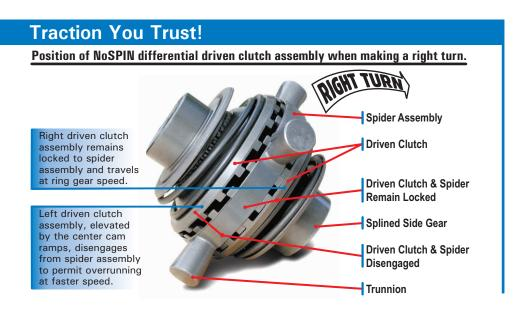
The Eaton NoSPIN is a speed sensitive automatic locking differential. It powers both drive wheels, yet automatically permits differential action to compensate for wheel speed differences that occur when making a turn or driving over obstacles.
