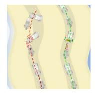
**Trailer Stability:** Counters unwanted oversteer in turns, shifting torque to the inside wheel
